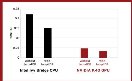
targetDP maps lattice-based parallelism to thread-level parallelism (TLP) and instruction-level parallelism (ILP). TLP maps to OpenMP threads on the CPU and CUDA threads on the GPU. The intelligent exposure of ILP has performance benefits for both CPUs and GPUs, as seen in the above graph which shows time for a binary collision LB computational kernel extracted from Ludwig.
