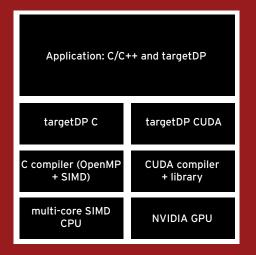
The lightweight targetDP framework consists of a set of C preprocessor macros, and a small C library interface for memory management.
