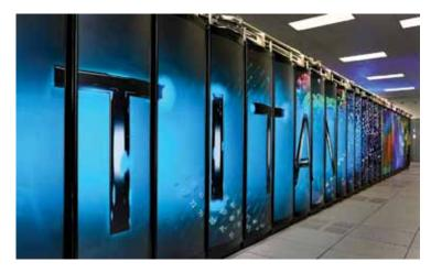
The simulations were performed on Titan at Oak Ridge National Laboratory, a Cray XK7 featuring 18,688 NVIDIA K20X GPUs
