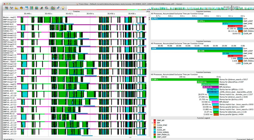
Figure 14: Performance visualisation of a hybrid version of Gromacs parallelized with MPI, OpenMP, and CUDA running on 8 nodes with 16 cores and 2 Nvidia K20 each. Every process uses one Nvidia graphic card and sends its kernels coloured in blue to two different streams.
