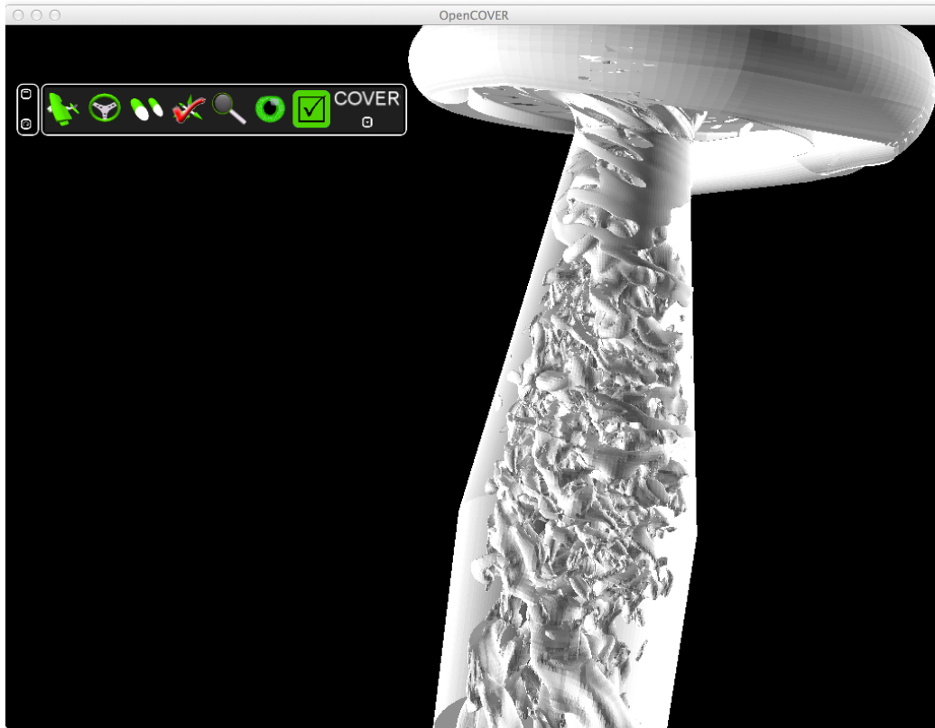
Figure 8: Iso surface and bounding geometry rendered in parallel on remote system together with local 3D menus.
