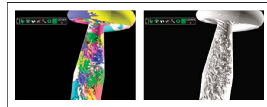
Figure 19: Contribution of nodes in different colours (left) and final composited image (right) of IHS pump turbine test case.
